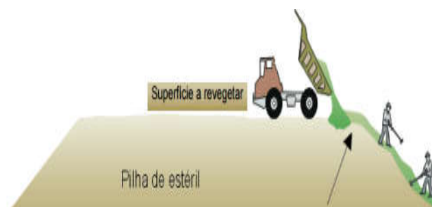
Figure 9- Placement of organic soil in the revegetative area
