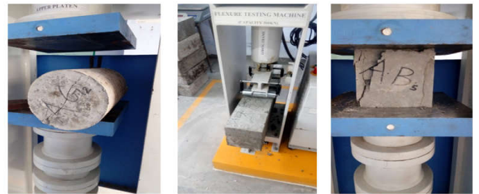
Figure 9 a) shows the testing of the cylindrical specimen b) shows the failure of the beam specimen c) shows the testing of the cubical specimen
