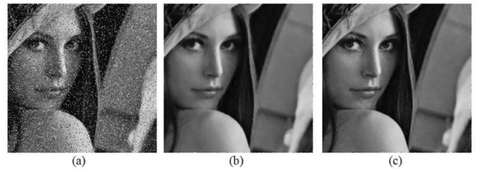
Figure 3 Example of filtering using FMF (a) image corrupted by impulsive noise (10%), (b) Noisy cleaning by first stage FMF, (c) edge sharpening by second stage filter.
