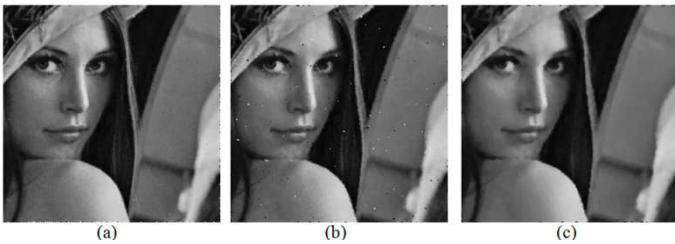
Figure 6 Results obtained by removing 20% impulsive noise using (a) proposed FMF, (b) 3X3 median filter, (c) 5X5 median filter.
