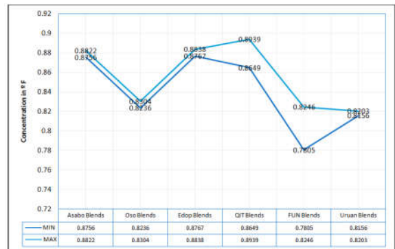
Figure 5 Graph Minimum and maximum values for specific gravity in different crude oil from Akwa Ibom State.
