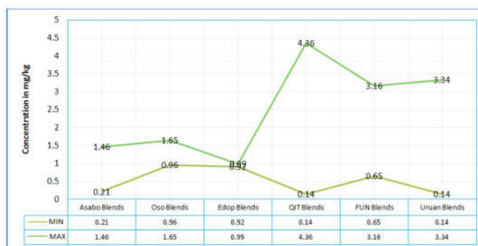
Figure 14 Graph Minimum and maximum values of cadmium in different crude oil from Akwa Ibom State.
