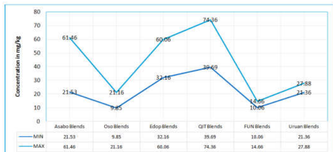
Figure 11 Graph Minimum and maximum values of iron in different crude oil from Akwa Ibom State.
