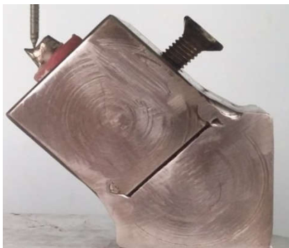
Figure 6 Tooth mounted on customized platform testing under universal testing machine
