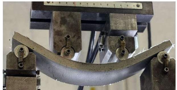
Fig 4 Flexure test on Slab
