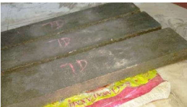
Fig 5 Casting of ECC Concrete Slab
