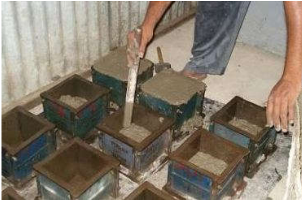
Fig 4 Casting of ECC Concrete Cube
