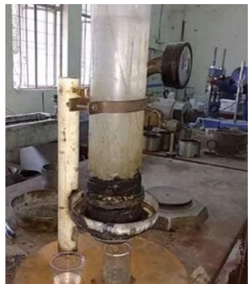
Figure 1 Permeametersketch (left) and actual (right)
