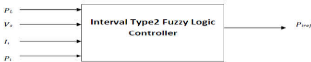
Fig 17 Structure of Type-2 FLC extended with four input values and one output value.
