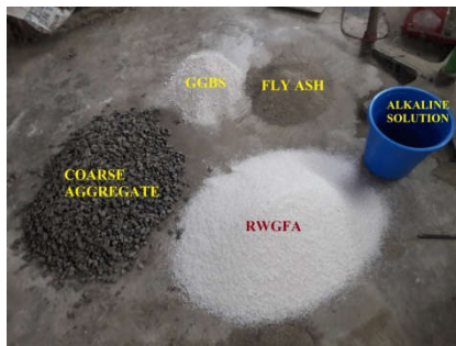
Figure 3 Materials used for RWGFA Geopolymer Concrete
