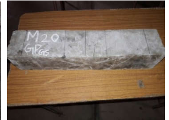
Figure 6 (c) Crack Patterns of Prism after testing
