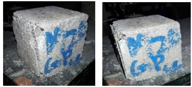
Figure 6 (a) Crack Patterns of Cubes after Testing
