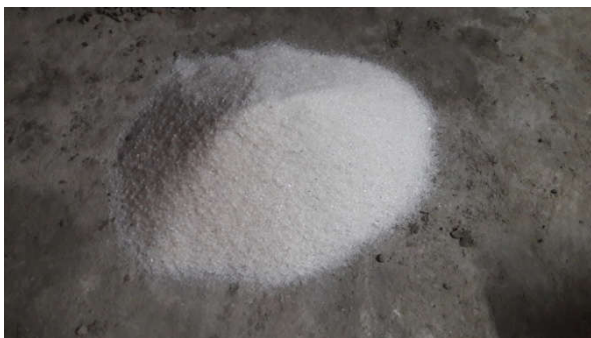
Figure 1 Recycled Waste Glass as Fine Aggregate
