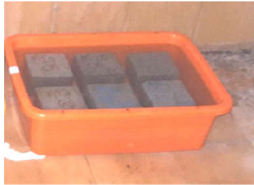
Figure 5 Specimens Immersed in MgSO 4 with Na 2 SO 4 Solution
