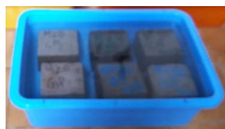
Figure 4 Specimens Immersed in HCl Solution
