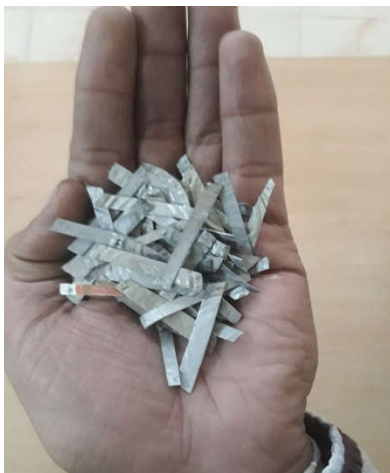
Fig 2.1 Fibres cut out from waste steel bottle caps
