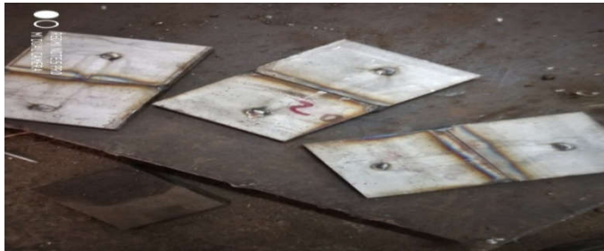
Fig 5 Butt Joint of SS202 and SS304 by TIG & MIG
