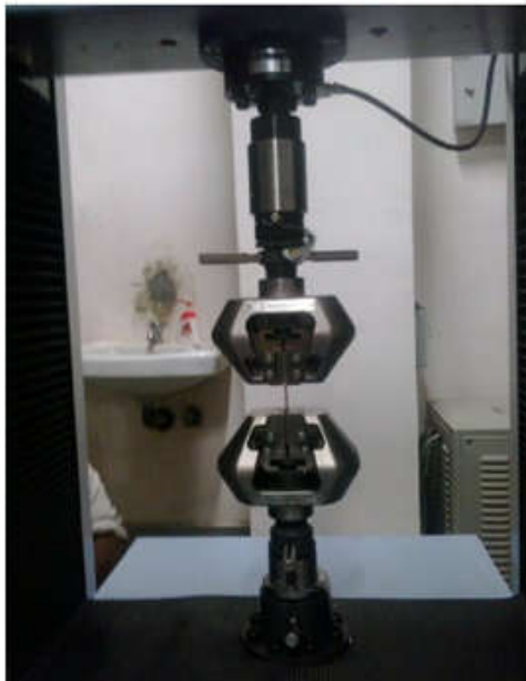
Fig 6 Specimen under the Tensile Test
