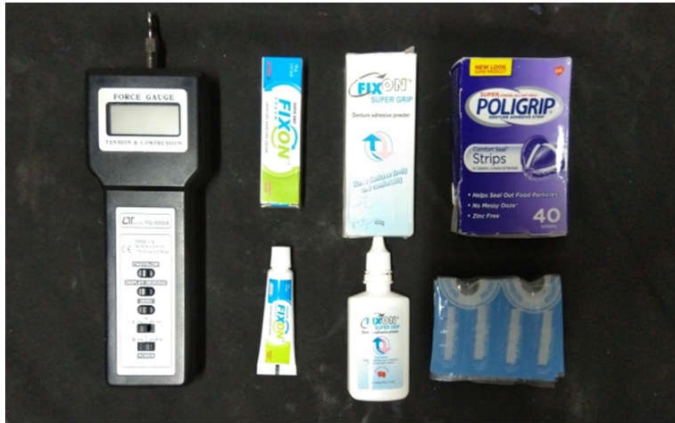
Fig 1 Materials used for testing retention of denture base and denture adhesives.
