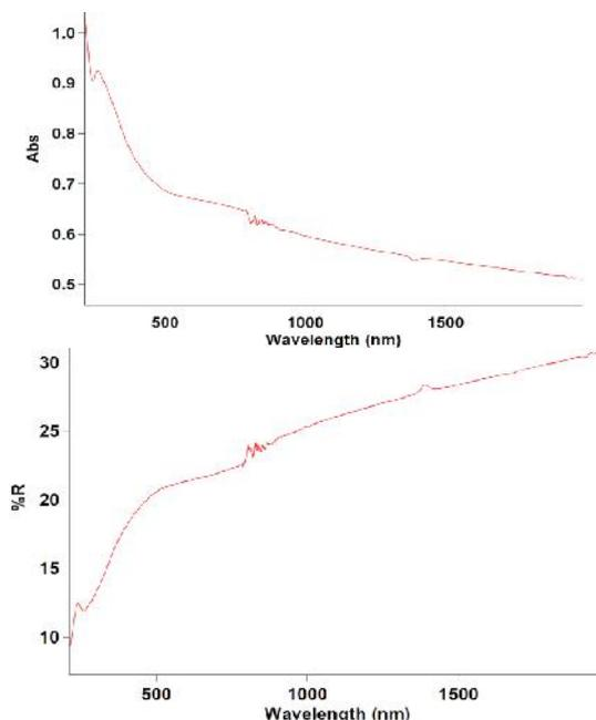
Figure1 UV-VIS spectrum of YSrBiCuO (a) Absorbance (b) reflectance
