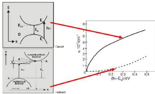
Fig.3 direct, indirect optical transition
