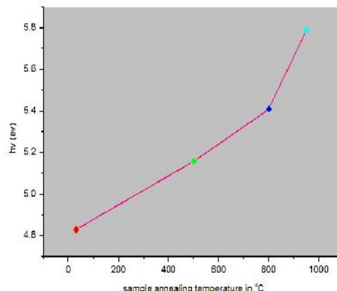
Fig.7 Band gap energy variation with the samples annealed at 30°C, 500°C, 800°C & 950°C of YSrBiCuO
