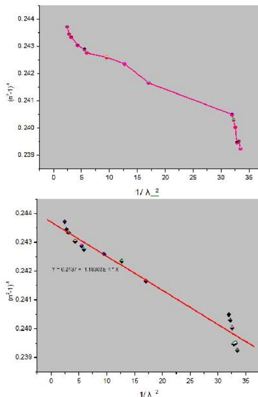
Fig.11  $(n^2-1)^{-1}$  versus  $1/\lambda^2$  curve (curve and linear fit)
