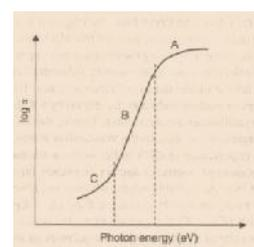
Fig.2optical band gap energy variation with absorption
