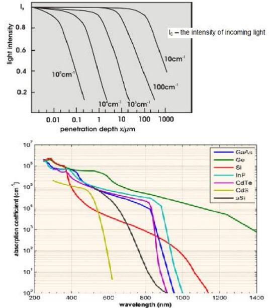
Fig.5 penetration depth plot related to absorption behaviour.
