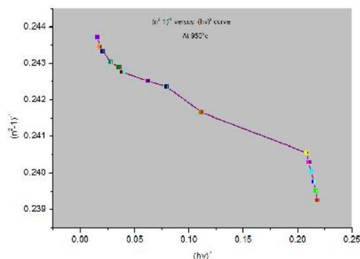
Fig.10  $(n^2-1)^{-1}$  versus  $(hv)^2$  curve. (YSrBiCuO)
