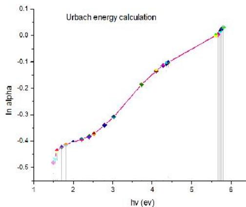
Fig.8 Absorption variation with photon energy of YSrBiCuO
