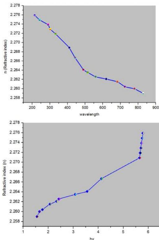
Fig.9 Variation of Refractive index (n) with wavelength and photon energy (YSrBiCuO).
