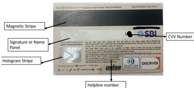
Figure 10 Standard Indian Debit Card with Overall security features (Back Side)
