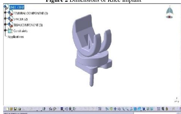
Figure 3 Assembly Model of Knee Prosthesis
