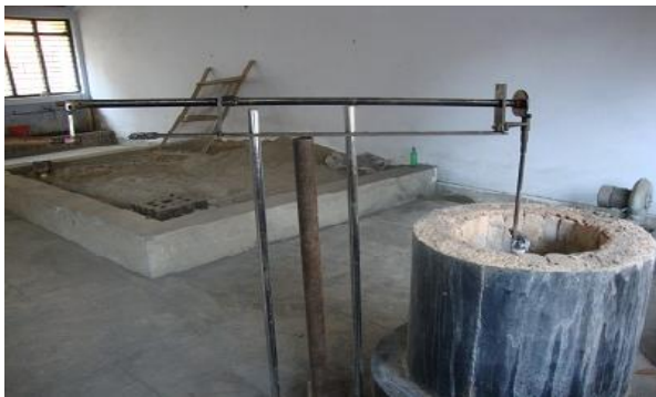
Open hearth furnace with stirring arrangement
