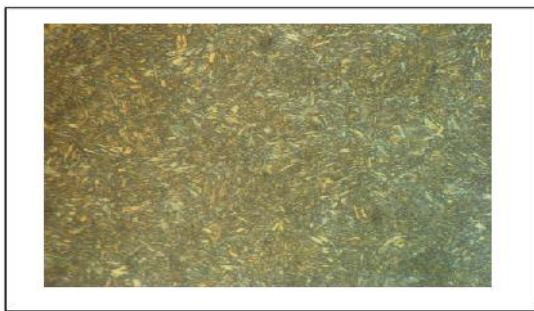
Figure.5 micrograph by M.O. (X50), in which the martensitic structure of a conventionally annealed steel is observed and water quenching.
