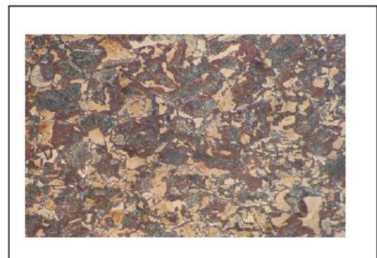
Figure.9 micrograph by M.O. (X50), in which a multiphase structure of the steel is observed DIN CK55, subcritical annealed at 750 ° C and oil quenching.
