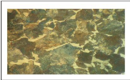
Figure.3 micrograph by M.O. (X100), where the reception structure of the steel is observed, hotworked and normalized.
