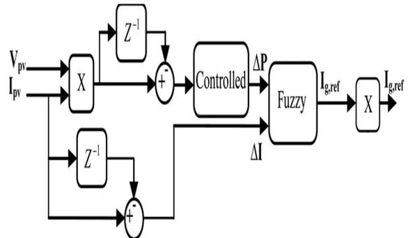
Figure 7 Block diagram of the FLC-based MPPT
