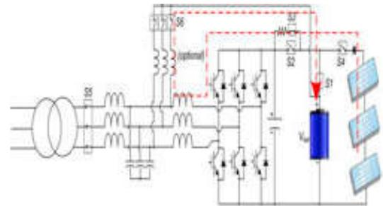
Figure 6 Mode 2—PV to battery
