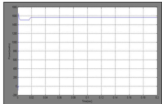
Figure 15 Output Power of the DC-DC Conversion
