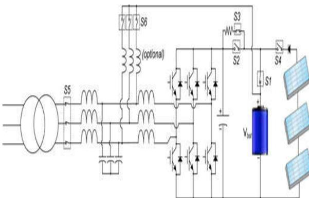
Figure 4 Schematic of the proposed RSC circuit
