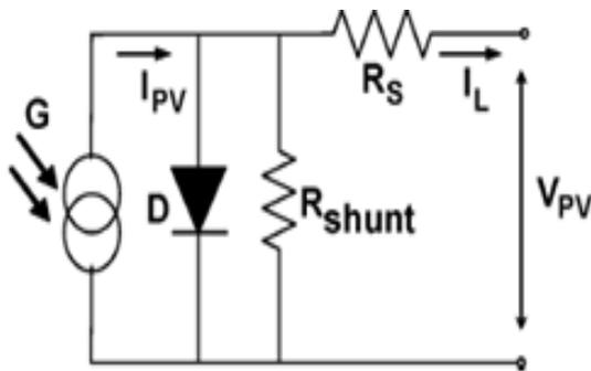
Figure 2 Equivalent circuit of a PV cell
