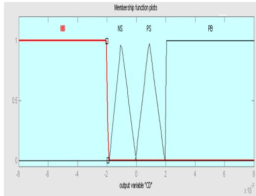
Figure 10 Membership function: Output  $\Delta D$
