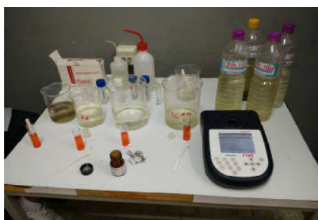
Figure 1 Testing the water samples of lake Hawassa by using Wagtech Photometer 7100
