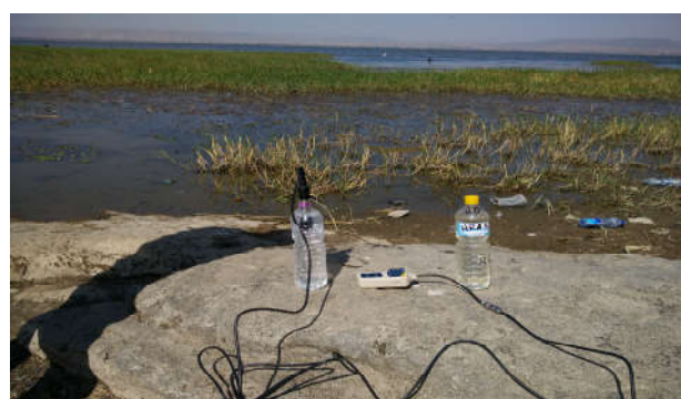
Figure 2 Testing Dissolved oxygen in the site by using Wagtech DO meter.
