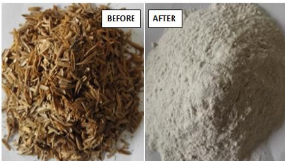
Plate 2 Rice husk sample (Before) and Polysilica Sample (After)
