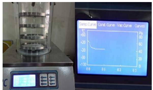
Plate 3 The Freeze Dryer and the Sample Curve Plot after Lyophilization Process
