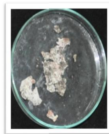
Plate 2 PHBV subjected to soil burial Assay
