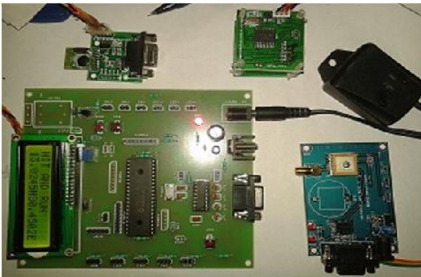
Fig.12 GPS tracks the location and the alert passed to server via zigbee
