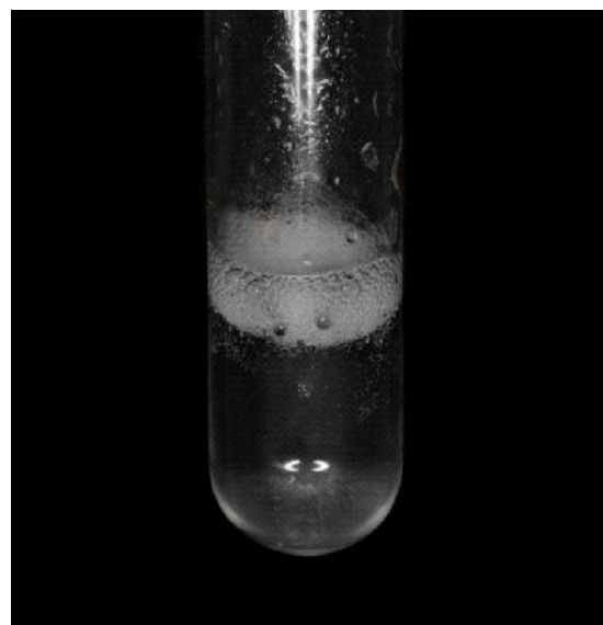
Figure 6 A white precipitate formed by mixing chlorhexidine with EDTA.
