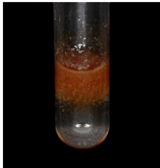
Figure 5 A brownish-orange precipitate formed by mixing chlorhexidine with sodium hypochlorite.
