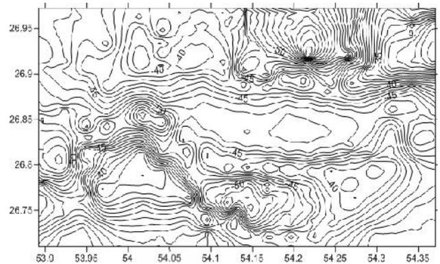
Figure 4 contour map. The complete Bouguer anomaly of the region with the density  $(2.6g/cm^3)$  and the balance distance 1 mm Gal; by using the Variogram's method
