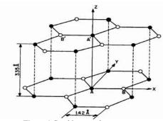
Figure 1 Graphite crystal structure
