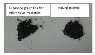
Figure 2 Comparison of appearances of synthesized expanded graphite and natural graphite
