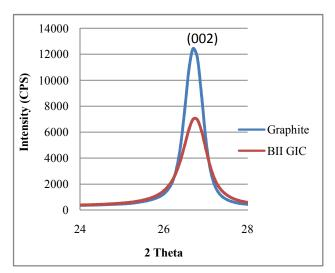
**Figure 4** XRD pattern of natural graphite and treated graphite
