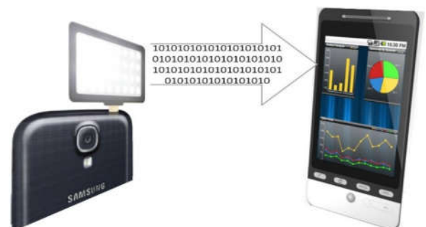
Figure 1 VLC applied to data transmission in mobiles
