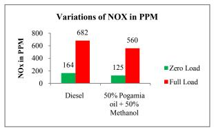
Fig-5 shows the variations of Nitrogen dioxide for Diesel and Pongamia oil blended with Methanol at Zero Load and Full Load
