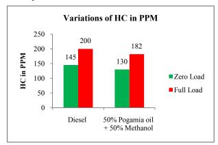
Fig.4 shows the variations of Unburnt Hydro Carbon for Diesel and Pongamia oil blended with Methanol at Zero Load and Full Load
