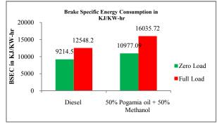
**Fig-2** shows the variations of Brake Specific Energy Consumption for Diesel and Pongamia oil blended with Methanol at Zero Load and Full
