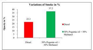
Fig-7 shows the variations of Smoke for Diesel and Pongamia oil blended with Methanol at Zero Load and Full Load
