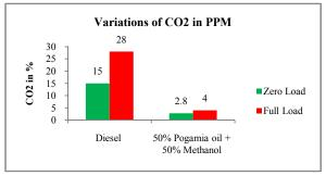
Fig-6 shows the variations of Carbon dioxide for Diesel and Pongamia oil blended with Methanol at Zero Load and Full Load
