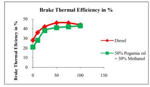
Fig-3 shows the variations of Brake Thermal Efficiency for Diesel and Pongamia oil blended with Methanol at different Loads
