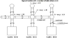
Figure 3: Layout diagram for circuit1
