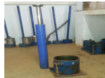
Fig.3 modified proctor apparatus
