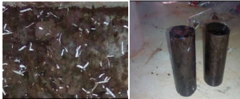
Fig 4 sample prepared by plastic strips.
