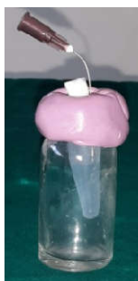
Fig1 Irrigant collection apparatus similar to that of Meyers and Montgomery
