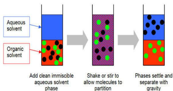
Figure 5 Liquid Liquid Extraction Mechanism
