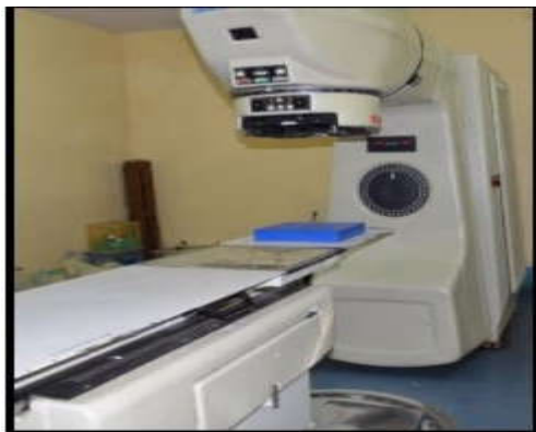
Figure2 Cobalt Irradiation Unit
