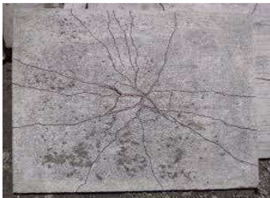
Fig 9 crack pattern during testing on slab
