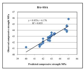
Figure 4 Comparison between predicted strength vs observed predicted strength on RBH & UPV
