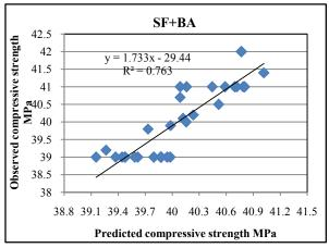
Figure 2 Comparison between predicted strength vs observed predicted strength on RBH & UPV
