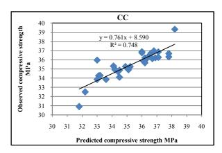
Figure 1 Comparison between predicted strength vs observed predicted strength on RBH & UPV
