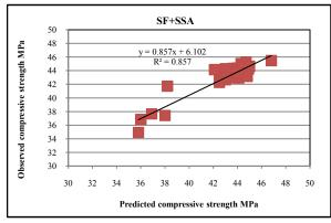
Figure 3 Comparison between predicted strength vs observed predicted strength on RBH & UPV
