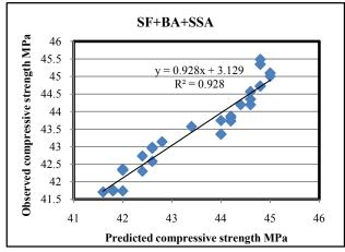
Figure 5 Comparison between predicted strength vs observed predicted strength on RBH & UPV
