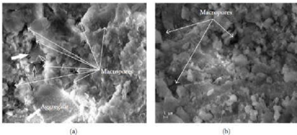
Figure 1 Reduction of porosity and therefore, permeability of concretes with Nano-silica; (a) concrete without Nano-silica; (b) concrete with Nano-silica (TorabianIsfahani *et al.*, 2016)
