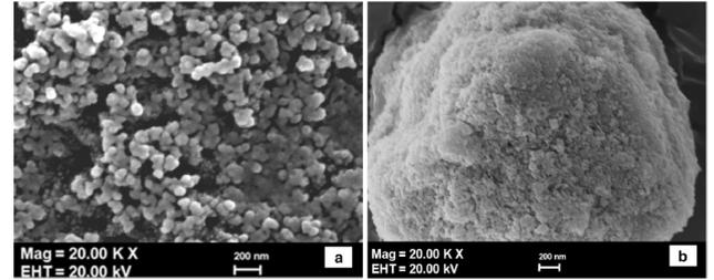
Figure 2 Powdered Nano-silica (a) and Colloidal Nano-silica (b) (Singh *et al.*, 2015)
