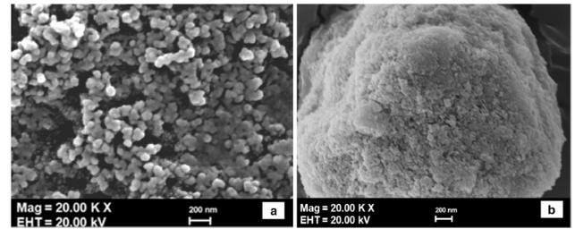
Figure 2 Powdered Nano-silica (a) and Colloidal Nano-silica (b) (Singh *et al.*, 2015)
