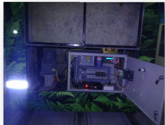
Figure 8 PLC based embedded system in the car in evolution of life Gallery
