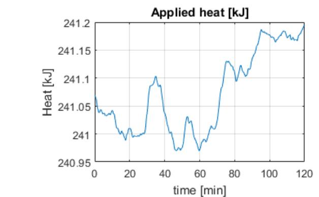
The next figure shows the heat disturbance in kJ. Note that the interruption changes by as much as half percent of the normal heat value.
