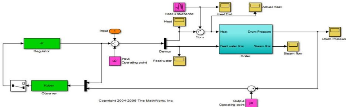
The boiler control model's pre-load function initializes the controller magnitude. It is important because to calculate the operation point and linear model, the MATLAB model must be run. Note that x0, z0 are set after the operation point computation and are thus initially set to zero. The viewer and manager are calculate at the controller plan step and are also initially set to zero.
