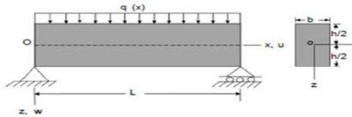
**Figure 1** Composite beam subjected to uniformly distributed load
