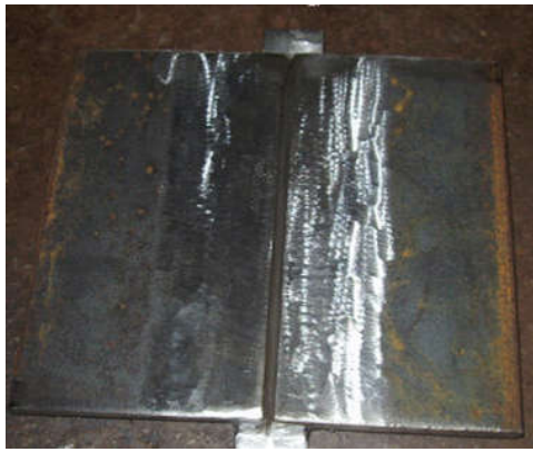
Figure 6 square butt joint (root gap - 2 mm)
