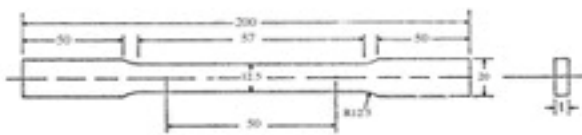
Figure 7 Standard tensile test specimen (ASTM E8-09)
