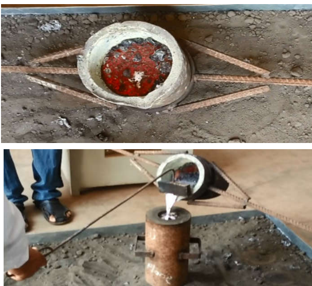
Figure 2 pouring of molten metal
