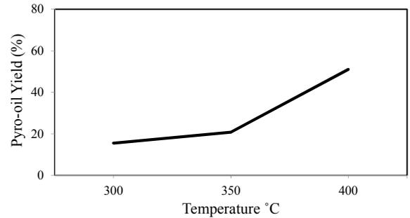
Figure 8 Variation of pyro-oil yield (%) versus temperature. Zeolite is used as catalyst
