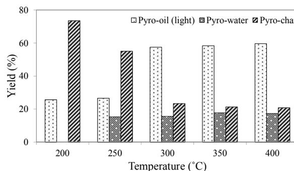
**Figure 3** Evolution of the pyro-products yield (%) versus temperature. Cu(NO<sub>3</sub>)<sub>2</sub> is used as catalyst
