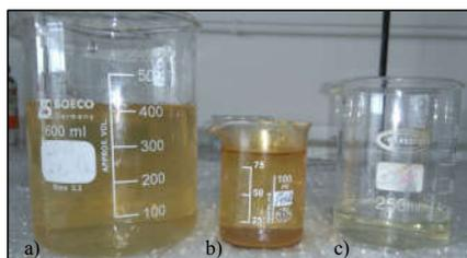
**Figure 2** Aqueous fraction treated by FeCl<sub>3</sub>: a) Before treatment, b) During treatment, and c) After treatment
