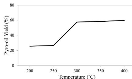
**Figure 4** Variation of pyro-oil yield (%) versus temperature. Cu(NO<sub>3</sub>)<sub>2</sub> is used as catalyst
