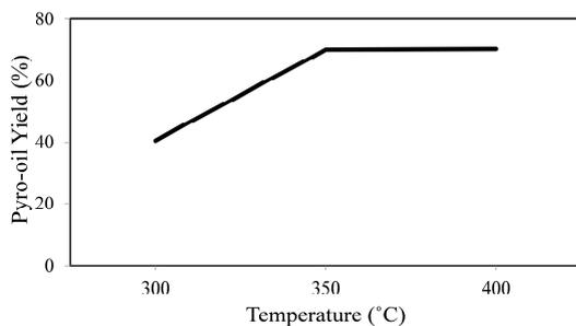
Figure 6 Variation of pyro-oil yield (%) versus temperature. Sodium hydroxide is used as catalyst
