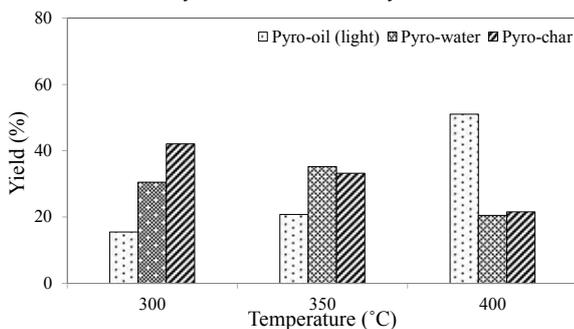
Figure 7 Evolution of the pyro-products yield (%) versus temperature. Zeolite is used as catalyst
