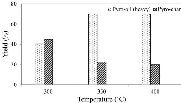
Figure 5 Evolution of the pyro-products yield (%) versus temperature. NaOH is used as catalyst
