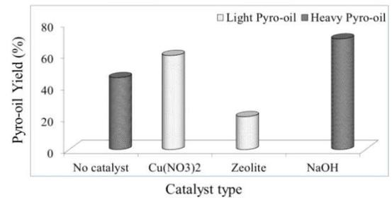
Figure 9 Variation of pyro-oil yield (%) versus type of catalyst
