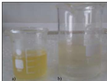
Figure 10 Pyro-water treatment by FeCl<sub>3</sub>: a) Before treatment, and b) After treatment
