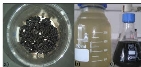
**Figure 1** Different fractions of diesel oil sludge: a) solid fraction, b) aqueous fraction, and c) oil fraction.
