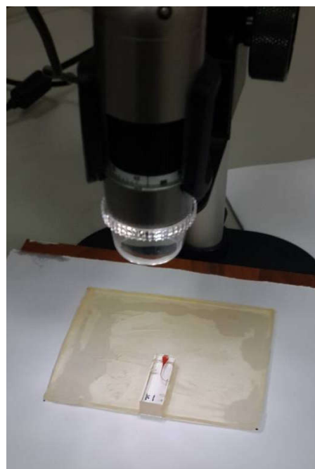
Figure 1 Digital microscope attached to Dino-Lite stand and placed at a fixed distance from the sample.
