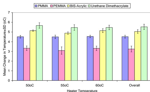
Fig 4 Graphical comparison of material temperature at different heater temperatures
