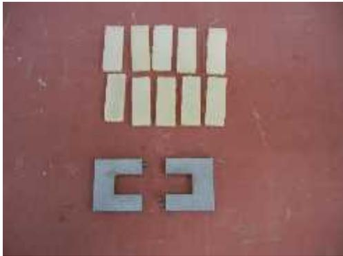
Fig 1 Stainless steel die and samples fabricated through it
