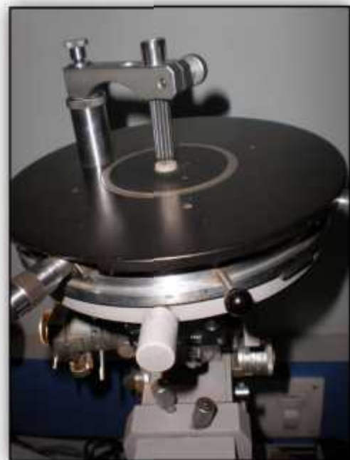
Fig. 3 Vickers Microhardness testing of sample
