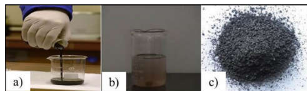
Figure 3 Different fractions of pyro-products: a) oil fraction, b) aqueous fraction and c) solid fraction.
