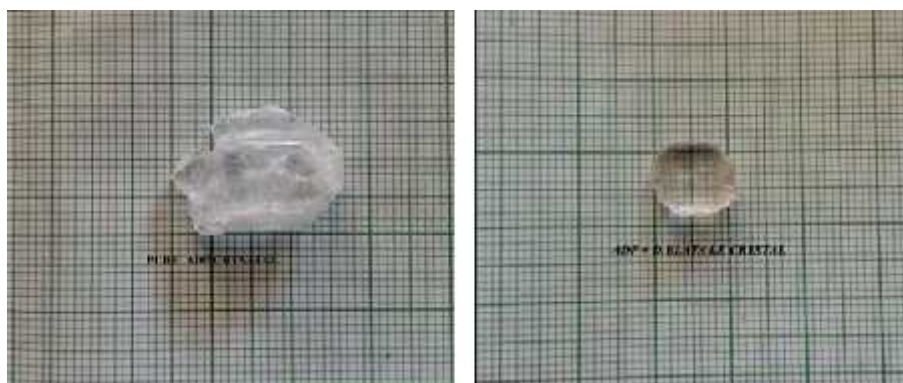
Fig 1 Photographs of the Pure ADP and Delonix elata leaf extract doped ADP Crystals
