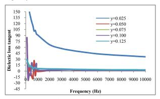
Figure 3 Variations of dielectric loss with frequency of  $Ni_{0.4}\,Mg_{0.4}\,Cd_{0.2}$   $Y_yFe_{2-y}O_4$  nanoferrites
