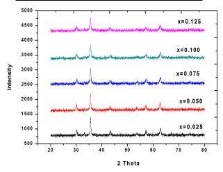
**Figure 1** Structural properties of  $Ni_{0.4}Mg_{0.4}Cd_{0.2}$   $Y_y$   $Fe_{2-y}O_4$  nanoferrites by XRD
