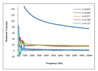
Figure 2 Variations of dielectric constant with frequency of  $Ni_{0.4}Mg_{0.4}$  $Cd_{0.2}Y_yFe_{2-y}O_4$  nanoferrites
