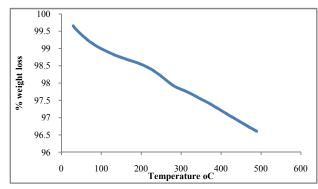
Figure 5 TGA curve for Ni<sub>0.4</sub> Mg<sub>0.4</sub> Cd<sub>0.2</sub> Y<sub>0.075</sub> Fe<sub>1.925</sub> O<sub>4</sub> nanoferrites
