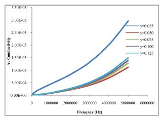
Figure 4 Variations of AC conductivity with frequency of  $Ni_{0.4} Mg_{0.4}$  $Cd_{0.2} Y_v Fe_{2-v} O_4$  nanoferrites
