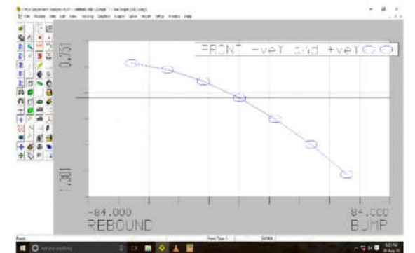
Fig: Toe Angle change in bump
