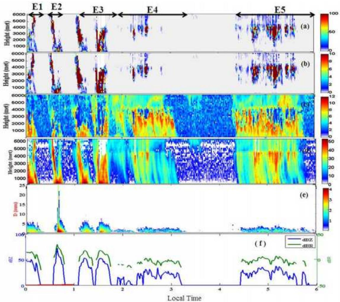
Figure 4 Typical Rain Integral parameters obtained from MRR and Parsivel Disdrometer on 22<sup>nd</sup> April 2010 during Hailstorm event.
