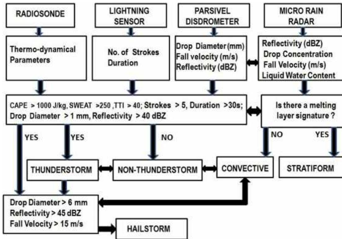
Figure 2 Algorithm for classification of mesoscale system into of Stratiform, mixed, convective, thunderstorm, non-thunderstorm, Hailstorm
