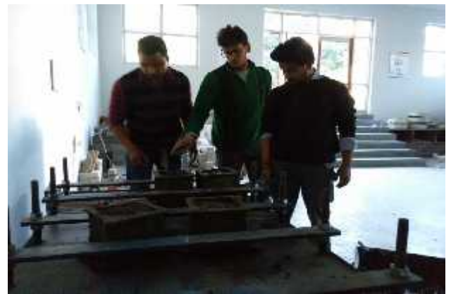
Figure 3 Compaction of concrete being done on the vibration table
