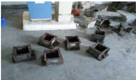
Figure 1 Cast iron moulds prepared for casting concrete cubes
