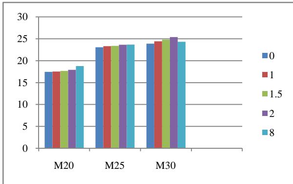
Figure 7 Graph showing increase in compressive strength for curing period of 7 days
