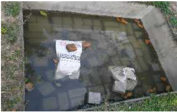
Figure 4 Cubes are being submerged in the curing pond for curing period of 7, 14 & 28 days
