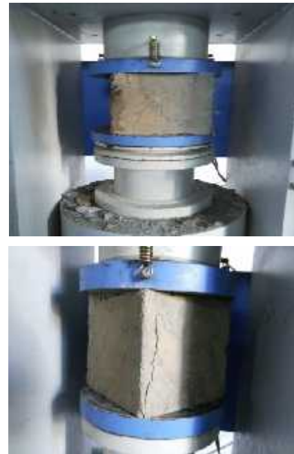
Figure 9 Conventional cube has multiple cracks (Left) & Fibre reinforced cube has a single crack (Right)
